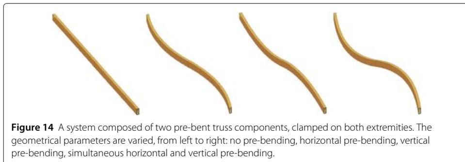
**Figure 14** A system composed of two pre-bent truss components, clamped on both extremities. The geometrical parameters are varied, from left to right: no pre-bending, horizontal pre-bending, vertical pre-bending, simultaneous horizontal and vertical pre-bending.
