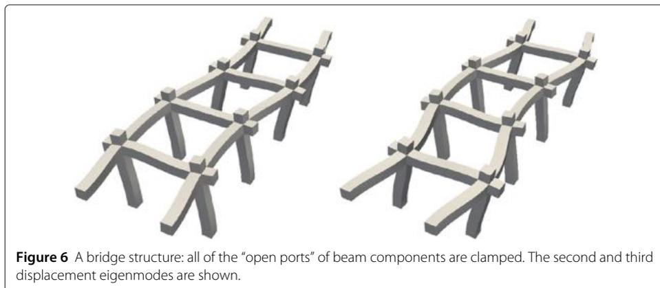
**Figure 6** A bridge structure: all of the “open ports” of beam components are clamped. The second and third displacement eigenmodes are shown.
